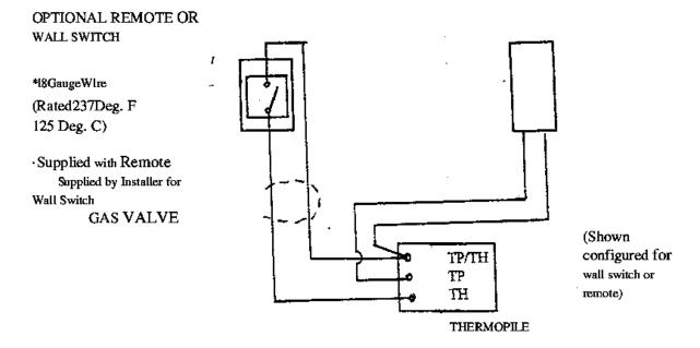
Note! Basket is delivered with Jumper wire installed. It must be removed for external switch or remote control to work.
