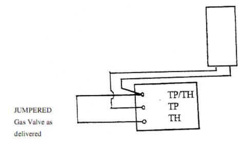
Remove factory jumper when installing remote control
