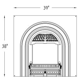
Note: the Windsor Arch without backing plate dimensions are 31"w (x) 34"h
