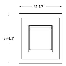
Note: the Ledge Front without backing plate dimensions are 27-3/8"w (x) 30"h
